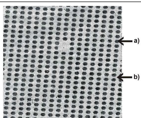
Fig. 1: Ellipsometric contrast image ( $0.4 \times 0.4 \text{ mm}^2$ ) of patterned polypeptide on gold. Arrows indicate two interesting „regions of interest“ (ROI) : a) the pattern with the grafted polypeptide (44 nm thick) and b) the space between them with loosely adsorbed poly-peptides (4 nm thick). [1]
